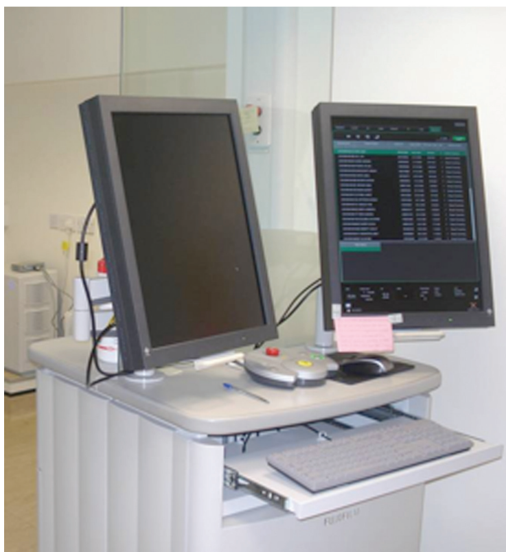
Figure 2 Workstation with colour monitor showing the worklist for the session (right) and monochrome monitor that displays the image on acquisition (left).
